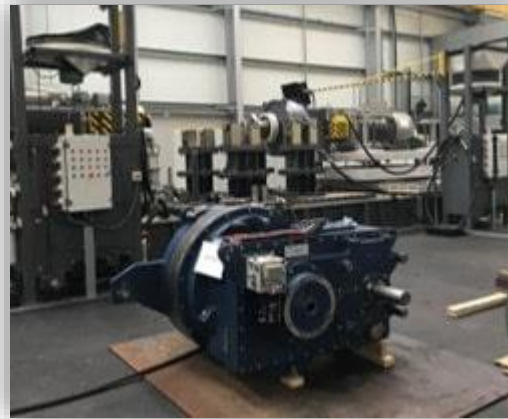
Test Bench for gearboxes up to 2,5 MW
