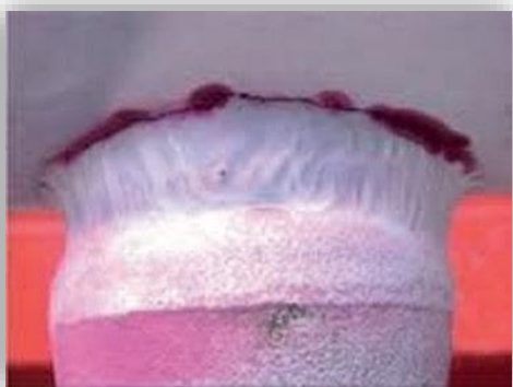
Liquid Penetrant Test
